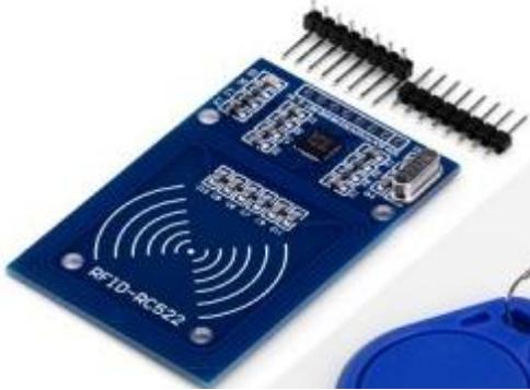
*Figure 13 - The MIFARE RFID reader – Image provided by Gear Best*
