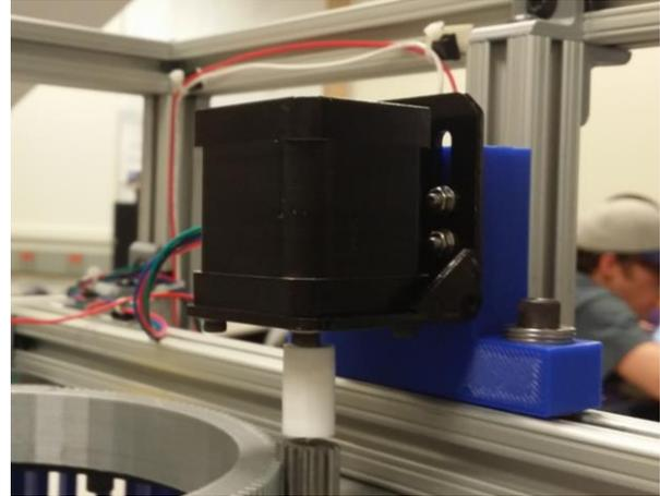
Figure 6 - The NEMA 17 stepper motor mounted in the DispensUM design, driving the rotary carousel
