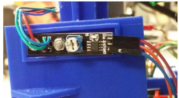
Figure 12 - The modified QTI sensor mounted onto the pill chute
