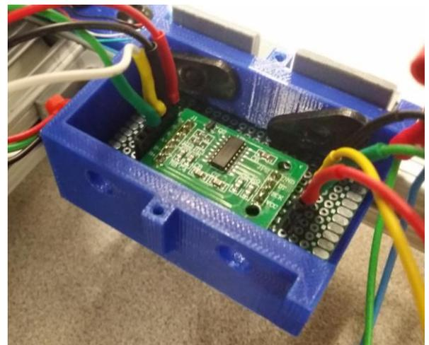
Figure 11 - The SMAKN HX711 weighing sensor
