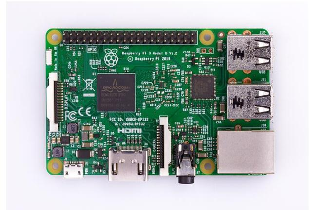
Figure 3 - The Raspberry Pi 3 Model B System on a Chip - image provided by Raspberry Pi Foundation
