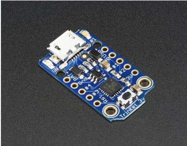
Figure 1 - The Adafruit Trinket Microcontroller – image provided by Adafruit
