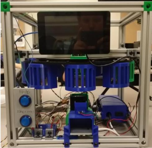
Figure 4 - The DispensUM design with the touchscreen mounted on the top and the help and dispense button located on the bottom left of the design
